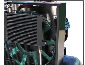
Air cooled after cooler on Elite unit
