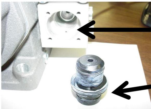
Inlet valve control Piston cylinder
