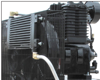
Air cooled after cooler Elite unit
