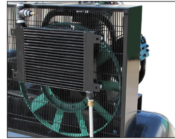
Air cooled after cooler Elite unit
