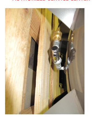
Once drain is clean, put screen, cap back in clean out and tighten cap
