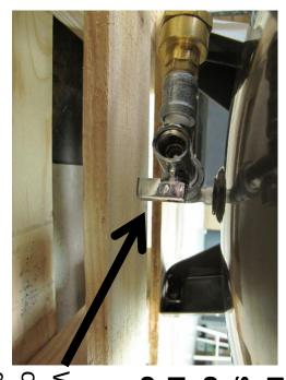
Note: Before this step make sure that you are not looking directly at drain opening air pressure and debris will come out of opening
