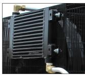
Air cooled after cooler on Elite unit
