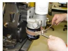
Detach the pilot air tube and the oil return tube
