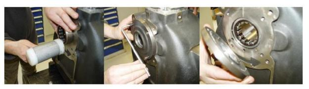
Insert the rotors carefully in the housing.
